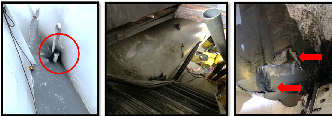
Figure 4. Left: Fuel tank vent pipe (soot residual from explosion), Center: Bulkhead between fuel tank and engine room (ballooned/ exploded), Right: Bulkhead penetrated (fractured from explosion); photographs taken by the Investigating Officer.
